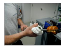
7. Slide the insert back into the strut body taking care not to roll the edge of the seal.
