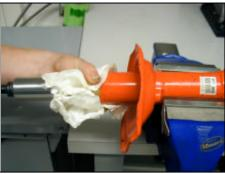
2. Remove the nut on the bottom of the strut tube.
