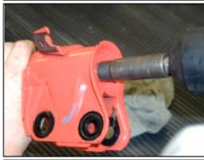
3. Withdraw the damper insert, being careful as the bump stop is pulled past the seal.
