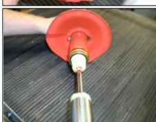
4. Put some of the grease carried on the bump stop around the retaining washer at the end of the rod. Pull and twist the bump stop off over the retaining washer. Use a cloth or tissue to provide a grip on the bump stop.
