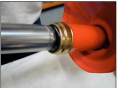
8. Rotate the insert when it reaches the bottom of the strut body until the flats on the threaded end drop through and locate in the hole.
